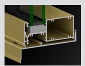
Designed to accept up to 44mm IGUs with 12mm bite. Pocket reducers can be used to reduce the glazing pocket dimensions so thinner IGUs can be accomodated
